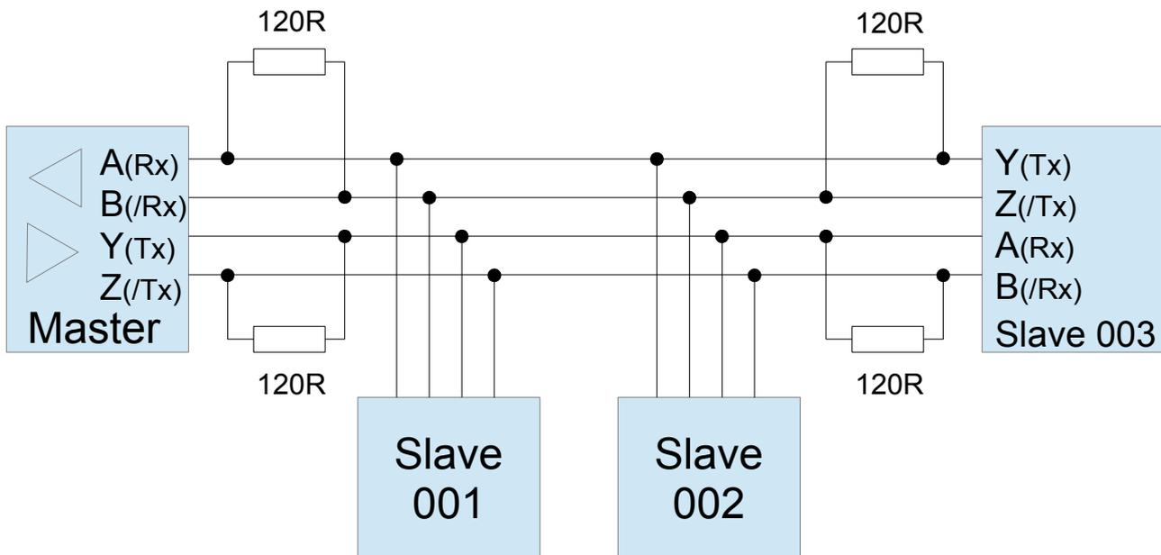
To minimise reflections, the line should be terminated at both ends in its characteristic impedance, and stub lengths off the main line should be kept as short as possible. The slew-rate-limited transceiver we use is more tolerant of imperfect termination. Nominal values for the termination resistors is 120 Ohms.
