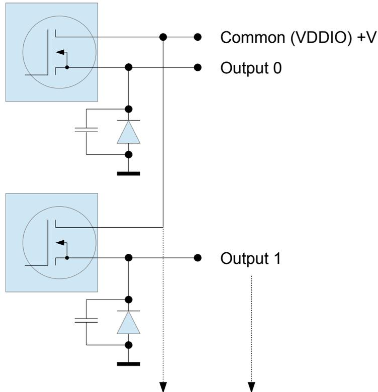
Should the drivers become accidentally reversed i.e. a negative voltage is applied to the drain with respect to the 0 volt rail, the diode will automatically conduct, clamping the maximum voltage to 0.7 of a volt with respect to ground, this prevents damage to the driver.
