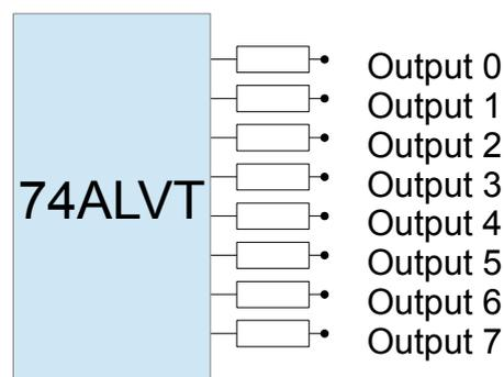
The output of the IC is connected via 33R resistors to limit noise and damage to the circuit. PMC outputs +/- 35mA @ 5V. This means that basic signals can be sent and LED's activated. If more voltage or current is required to say drive a relay then drivers 8+ can be used; see following section.
