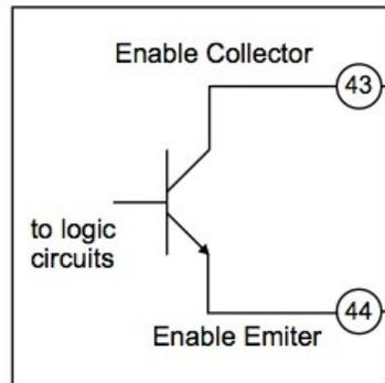
Please note that if there is a requirement to enable more than 2 drives in parallel the output will need to be buffered. This is due to the fact that most drives use an opto-isolated input that will need around 10mA to activate. TRM can supply a 4 output module to convert this if required which can be easily mounted on DIN rail.
